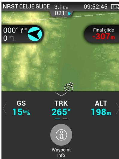
In the left part of the screen, standard wind information can be read. The Arrow shows the course of the wind in regards to the glider, the degrees of its direction from the North and the speed is shown below.
