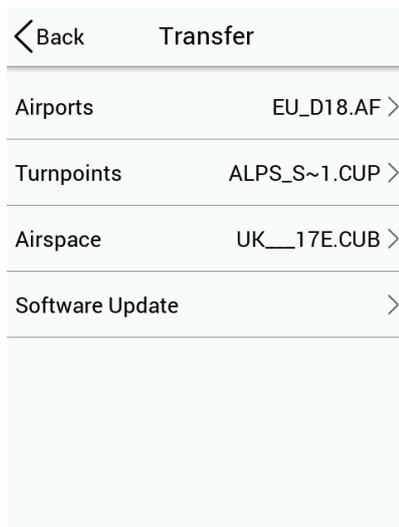
The transfer page is used for transferring turnpoint and task files (.cup), airport files (.af), airspace files (.cub) and software updates (.lxu). It is also used for selecting active files and deleting old files.
