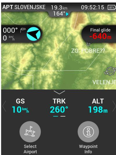
In the bottom of the screen, there is a configurable row of navboxes. In order to find out how they are configured, check ‘2.1 Vario page’.
