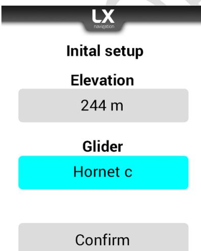
Initial setup appears every time the device is powered on. It consists of two essential pieces of information:
