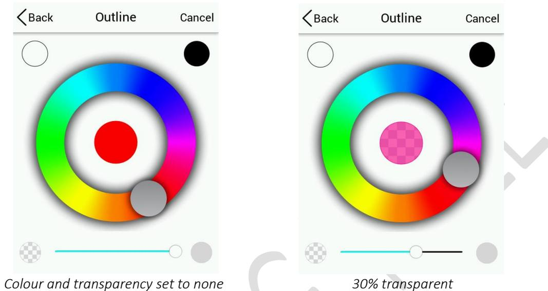
In general, when exiting a setup menu page, after making a change, selecting the '< Back' option in the upper left corner will save this setting, and selecting 'Cancel' will disregard the change you've made and keep the old setting.
