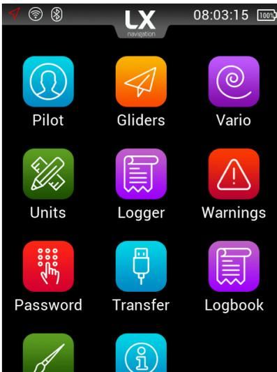
By swiping left on main vario page you get to the setup page. Under setup, the pilot can set all parameters of the unit. The menus are following:
